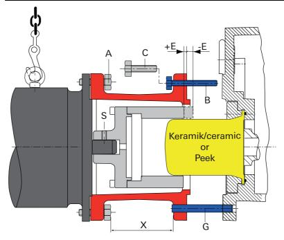
Fig. 4: Assembling drive motor with pre-assembled lantern
