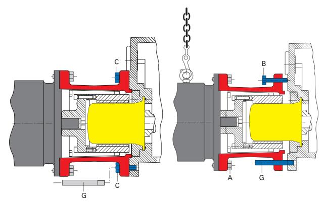
Fig. 1: Dismantling motor and lantern
