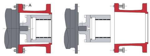
Fig. 2: Dismantling lantern
