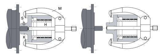
Fig. 3: Extracting the coupling half
